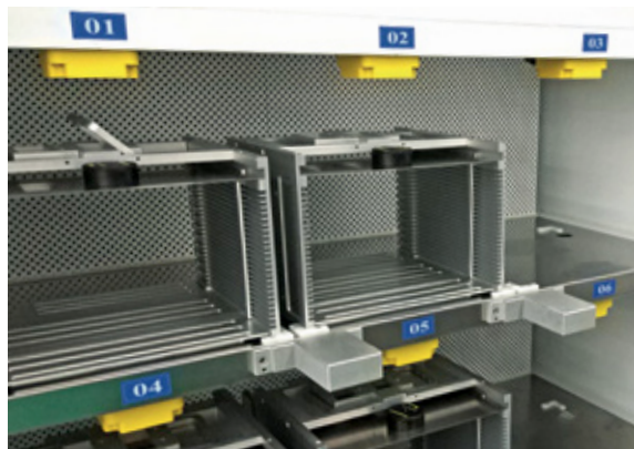
The RFID HF read/write heads on the top of the material racks read out the tags of the wafer carriers during stock placement and stock removal
